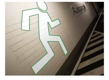
**Preco Line EP 2K NightLine** is a 2-component, thin-layer marking with luminescent properties and is used on asphalt and concrete surfaces. The marking was tested according to DIN 67510 Part 1, Class A (see BAM [German Federal Institute for Materials Research and Testing] report: 8.6E0024, sample no. 01 (b)). With a 0.6 mm coating, the following decay time was measured by BAM:
