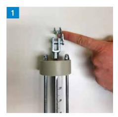
Fasten the cylinder: The cylinder is fastened to the mount by inserting the retaining bolt through the opening. The tension spring is then pushed down again.
