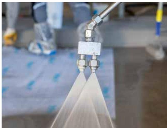
The double and a single nozzles are easy to interchange, and spare nozzles plus a nozzle extension are provided in addition. To prevent the nozzles from clogging with cured material after using Triflex SAM, they are placed in a container with Triflex cleaner, which is also supplied.
