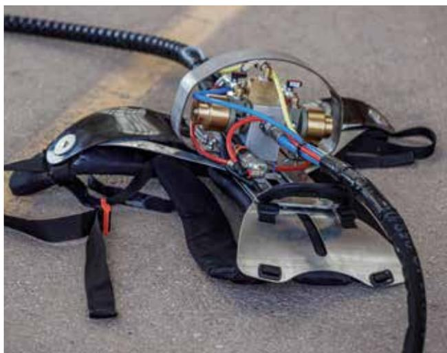
Outside the mobile unit, the mixing element and spray gun, including the selected nozzle, are used. The mixing unit is connected to the mobile unit by a hose, which contains five feed lines for conveying the following components from the machine to the mixing unit:
